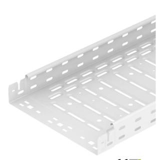
Cable tray with integrated quick fastening system. Continuous side perforations of 7 x 20 mm for the installation of additional connection and mounting components. With 11 mm perforation in the base for direct threaded rod suspension. Usable length 3,000 mm.
