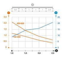
Load diagram, cable tray, type RKSM 60
