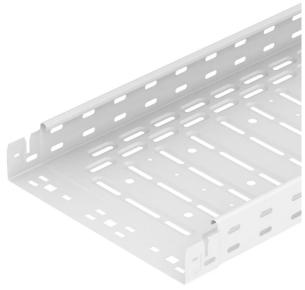
Cable tray with integrated quick fastening system. Continuous side perforations of 7 x 20 mm for the installation of additional connection and mounting components. With 11 mm perforation in the base for direct threaded rod suspension. Usable length  $3{,}000$  mm.
