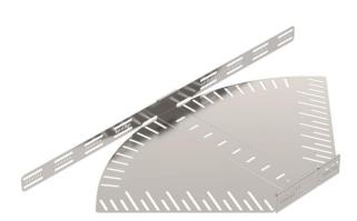
Angle-adjustable bend for the creation of a horizontal branch, fitting for lock and screw-on cable trays of side height 60 mm. Adjustable angle  $0-90^\circ$ . Screwless mounting with double clamps or screw connection with FRS truss-head screws and M6 combination nuts. Can be used indoors and outdoors. Fastening material must be ordered separately.
