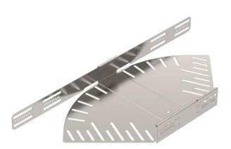
Angle-adjustable bend for the creation of a horizontal branch, fitting for lock and screw-on cable trays of side height 60 mm. Adjustable angle 0–90°. Screwless mounting with double clamps or screw connection with FRS truss-head screws and M6 combination nuts. Can be used indoors and outdoors. Fastening material must be ordered separately.
