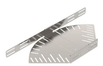
Angle-adjustable bend for the creation of a horizontal branch, fitting for lock and screw-on cable trays of side height 60 mm. Adjustable angle  $0-90^\circ$ . Screwless mounting with double clamps or screw connection with FRS truss-head screws and M6 combination nuts. Can be used indoors and outdoors. Fastening material must be ordered separately.
