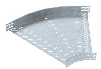
45° bend for the creation of a horizontal branch, fitting for lock and screw-on cable trays of side height 60 mm. Screwless mounting with double clamps or screw connection with FRS truss-head screws and M6 combination nuts. Can be used indoors and outdoors. Fastening material must be ordered separately.
