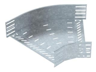
45° bend for the creation of a horizontal branch, fitting for lock and screw-on cable trays of side height 110 mm. Screwless mounting with double clamps or screw connection with FRS truss-head screws and M6 combination nuts. Can be used indoors and outdoors. Fastening material must be ordered separately.
