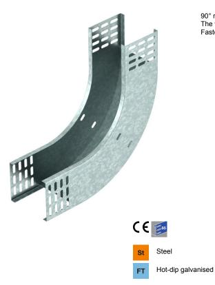
90° rising vertical bend, for all cable tray types of 85 mm side height. The vertical bend is pushed over the end of the cable tray and screwed tight. Fastening materials should be ordered separately.
