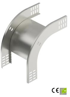
90° vertical bend, falling, for all cable tray types of 60 mm side height. The vertical bend is pushed over the end of the cable tray and screwed tight. Fastening materials should be ordered separately.
