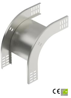
90° vertical bend, falling, for all cable tray types of 60 mm side height. The vertical bend is pushed over the end of the cable tray and screwed tight. Fastening materials should be ordered separately.
