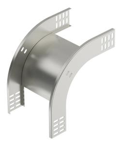
90° vertical bend, falling, for all cable tray types of 60 mm side height. The vertical bend is pushed over the end of the cable tray and screwed tight. Fastening materials should be ordered separately.
