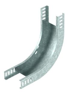
90° rising vertical bend, for all cable tray types of 35 mm side height. The vertical bend is pushed over the end of the cable tray and screwed tight. Fastening materials should be ordered separately.
