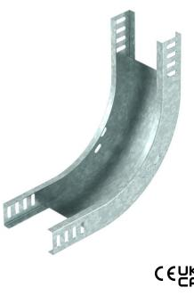
90° rising vertical bend, for all cable tray types of 35 mm side height. The vertical bend is pushed over the end of the cable tray and screwed tight. Fastening materials should be ordered separately.
