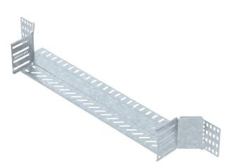
Add-on tee for the creation of a horizontal branch or cross-over, fitting for lock and screw-on cable trays of side height 110 mm. Screwless mounting with double clamps or screw connection with FRS truss-head screws and M6 combination nuts. Can be used indoors and outdoors. Fastening material must be ordered separately.
