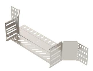
Add-on tee for the creation of a horizontal branch or cross-over, fitting for lock and screw-on cable trays of side height 110 mm. Screwless mounting with double clamps or screw connection with FRS truss-head screws and M6 combination nuts. Can be used indoors and outdoors. Fastening material must be ordered separately.
