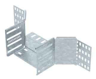
Add-on tee for the creation of a horizontal branch or cross-over, fitting for lock and screw-on cable trays of side height 110 mm. Screwless mounting with double clamps or screw connection with FRS truss-head screws and M6 combination nuts. Can be used indoors and outdoors. Fastening material must be ordered separately.
