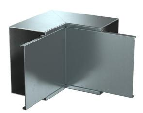
Internal corner with intumescent fire protection mesh for PYROLINE® Rapid PLM installation duct. Suitable for direct wall and ceiling mounting, mounting below system floors and on support systems. Tool-free joint mounting with PLM SI joint connector. The cover is snapped on without tools, allowing rapid inspection and retroassignment. The cover overhang allows offset cover mounting for continuous equipotential bonding of the entire duct section.
