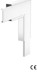
Flat angle with intumescent fire protection mesh for PYROLINE® Rapid PLM installation duct. Suitable for direct wall and ceiling mounting, mounting below system floors and on support systems. Tool-free joint mounting with PLM SI joint connector. The cover is snapped on without tools, allowing rapid inspection and retroassignment. The cover overhang allows offset cover mounting for continuous equipotential bonding of the entire duct section.
