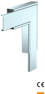
Flat angle with intumescent fire protection mesh for PYROLINE® Rapid PLM installation duct. Suitable for direct wall and ceiling mounting, mounting below system floors and on support systems. Tool-free joint mounting with PLM SI joint connector. The cover is snapped on without tools, allowing rapid inspection and retroassignment. The cover overhang allows offset cover mounting for continuous equipotential bonding of the entire duct section.
