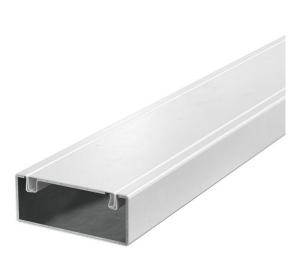
Metal installation duct with intumescent fire protection mesh for fireproof routing of cables. Classified as an installation duct El30, El60 and El90 according to EN 13501-2, tested according to EN 1366-5. The duct prevents the fire spread for the classified period of time, offering protection against the effects of a cable fire.
