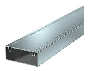
Metal installation duct with intumescent fire protection mesh for fireproof routing of cables. Classified as an installation duct El30, El60 and El90 according to EN 13501-2, tested according to EN 1366-5. The duct prevents the fire spread for the classified period of time, offering protection against the effects of a cable fire.
