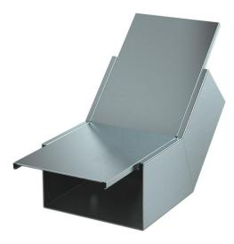
45° vertical bend, rising version, with intumescent fire protection mesh for PYRO-LINE® Rapid PLM installation duct. Suitable for direct wall and ceiling mounting, mounting below system floors and on support systems. Tool-free joint mounting with PLM SI joint connector. The cover is snapped on without tools, allowing rapid inspection and retroassignment. The cover overhang allows offset cover mounting for continuous equipotential bonding of the entire duct section.
