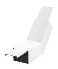
45° vertical bend, rising version, with intumescent fire protection mesh for PYRO-LINE® Rapid PLM installation duct. Suitable for direct wall and ceiling mounting, mounting below system floors and on support systems. Tool-free joint mounting with PLM SI joint connector. The cover is snapped on without tools, allowing rapid inspection and retroassignment. The cover overhang allows offset cover mounting for continuous equipotential bonding of the entire duct section.
