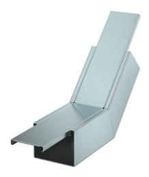
45° vertical bend, rising version, with intumescent fire protection mesh for PYRO-LINE® Rapid PLM installation duct. Suitable for direct wall and ceiling mounting, mounting below system floors and on support systems. Tool-free joint mounting with PLM SI joint connector. The cover is snapped on without tools, allowing rapid inspection and retroassignment. The cover overhang allows offset cover mounting for continuous equipotential bonding of the entire duct section.
