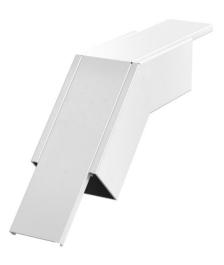
45° vertical bend, falling version, with intumescent fire protection mesh for PY-ROLINE® Rapid PLM installation duct. Suitable for direct wall and ceiling mounting, mounting below system floors and on support systems. Tool-free joint mounting with PLM SI joint connector. The cover is snapped on without tools, allowing rapid inspection and retroassignment. The cover overhang allows offset cover mounting for continuous equipotential bonding of the entire duct section.
