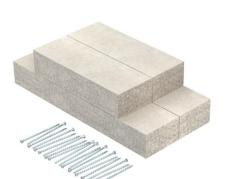
Wall connection collar for PYROLINE® Con S El60 fire protection duct, type PLCS D060810, consisting of fibre-glass light concrete, which is resistant to water and frost, for mounting on the fire protection duct in the area of wall connections and wall penetrations. Consists of 4 single plates (width 50 mm, depth 30 mm).
