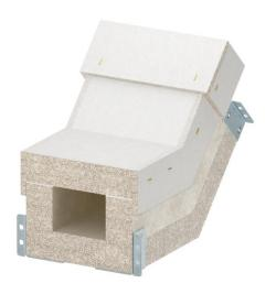
Vertical bend, rising, for PYROLINE® Con S El90 fire protection duct, type PLCS D090810, consisting of fibreglass light concrete which is resistant to water and frost for the creation of vertical changes of direction (45°) of the duct. Mounted connectors ensure quick mounting in situ, whilst loosely placed covers ensure quick inspection and reassignment.
