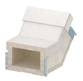
Vertical bend, rising, for PYROLINE® Con S El60 fire protection duct, type PLCS D061220, consisting of fibreglass light concrete which is resistant to water and frost for the creation of vertical changes of direction (45°) of the duct. Mounted connectors ensure quick mounting in situ, whilst loosely placed covers ensure quick inspection and reassignment.
