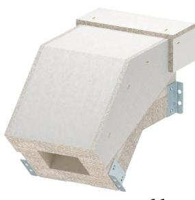
Vertical bend, falling, for PYROLINE® Con S EI90 fire protection duct, type PLCS D090810, consisting of fibreglass light concrete which is resistant to water and frost for the creation of vertical changes of direction (45°) in the duct. Mounted connectors ensure quick mounting in situ, whilst loosely placed covers ensure quick inspection and reassignment.
