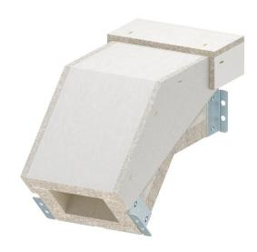
Falling vertical bend for PYROLINE® Con S El60 fire protection duct, type PLCS D060810, consisting of fibreglass light concrete which is resistant to water and frost for the creation of vertical changes of direction (45°) in the duct. Mounted connectors ensure quick mounting in situ, whilst loosely placed covers ensure quick inspection and reassignment.
