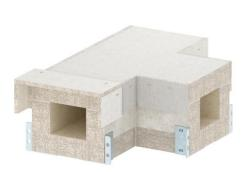
T piece for PYROLINE® Con S EI90 fire protection duct, type PLCS D090810, consisting of fibreglass light concrete which is resistant to water and frost, for the creation of T branches in the duct route. Mounted connectors ensure quick mounting in situ, whilst loosely placed covers ensure quick inspection and reassignment.
