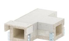
T piece for PYROLINE® Con S El60 fire protection duct, type PLCS D060810, consisting of fibreglass light concrete which is resistant to water and frost, for the creation of T branches in the duct route. Mounted connectors ensure quick mounting in situ, whilst loosely placed covers ensure quick inspection and reassignment.
