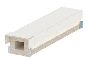
Fire protection duct made of water and frost-resistant fibreglass lightweight concrete of material class A1 according to EN 13501-1 for fireproof routing of cables in escape and rescue routes. El60 classification as installation duct according to EN 13501-2 on the basis of tests according to EN 1366-5. When there is an internal fire load (cable fire), the duct prevents the spread of fire from one fire section to another.
