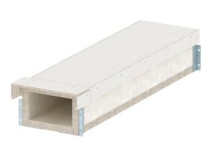
Fire protection duct made of water and frost-resistant fibreglass lightweight concrete of material class A1 according to EN 13501-1 for fireproof routing of cables in escape and rescue routes. El30 - El60 classification as installation duct according to EN 13501-2 on the basis of tests in accordance with EN 1366-5. When there is an internal fire load (cable fire), the duct prevents the spread of fire from one fire section to another.
