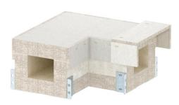
90° bend for PYROLINE® Con S El90 fire protection duct, type PLCS D090810, consisting of fibreglass light concrete which is resistant to water and frost for the creation of horizontal changes of direction in the duct. Mounted connectors ensure quick mounting in situ, whilst loosely placed covers ensure quick inspection and reassignment.
