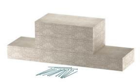
Wall connection collar for PYROLINE® Con D El90 fire protection duct, type PLCD D091220, consisting of fibreglass light concrete, which is resistant to water and frost, for mounting on the fire protection duct in the area of wall and ceiling connections and wall and ceiling penetrations. Consists of 3 single plates (width 100 mm, depth 40 mm). Including countersunk head screws. Including counter-sunk head screws.
