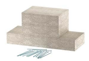
Wall connection collar for PYROLINE® Con D El90 fire protection duct, type PLCD D090810, consisting of fibreglass light concrete, which is resistant to water and frost, for mounting on the fire protection duct in the area of wall and ceiling connections and wall and ceiling penetrations. Consists of 3 single plates (width 100 mm, depth 40 mm). Including countersunk head screws. Including counter-sunk head screws.
