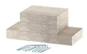
Wall connection collar for PYROLINE® Con D El60 fire protection duct, type PLCD D060810 consisting of fibreglass light concrete, which is resistant to water and frost, for mounting on the fire protection duct in the area of wall and ceiling connections and wall and ceiling penetrations. Consists of 3 single plates (width 100 mm, depth 30 mm). Including countersunk head screws.
