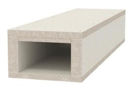
Fire protection duct made of water and frost-resistant fibreglass lightweight concrete of material class A1 according to EN 13501-1 for fireproof routing of cables in escape and rescue routes. El60 classification as installation duct according to EN 13501-2 on the basis of tests according to EN 1366-5. When there is an internal fire load (cable fire), the duct prevents the spread of fire from one fire section to another.
