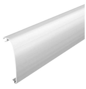
Trunking cover to create a design device installation trunking of the GAD series. "Soft" design version for complete coverage of the system opening and the switching and plug-in devices. The GAD OTA cover adapters are essential and must be planned on the trunking section with a max. spacing of 50 cm. A GAD OTD spacer must be placed between the trunking covers.
