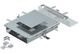
Ready-to-mount trunking extension unit with a device installation lid for the installation of a flush-mount unit of nominal size 9, consisting of the trunking base (floor trough with side and floor covering contact profiles), trunking lid with blank mounting opening and a flushfloor end cover. The scope of delivery contains 3 height-adjustable fixing brackets, 3 screed anchors, 1 lid butt support and 1 construction set for 90° angle.
