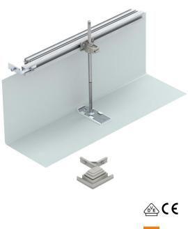
For the construction-side creation of a trunking junction as a 90° angle, T-piece or crossing. A flushfloor end cover is also required for the creation of a 90° angle (order separately). Suitable for the OKA-G and OKA-W trunking systems.
