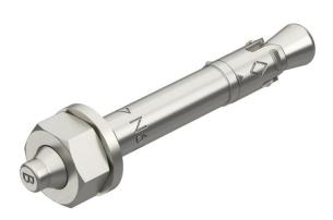
The nail anchor N can be used for multiple fastenings of non-load-bearing systems, indoors and outdoors, in cracked and non-cracked concrete, thereby combining the benefits of a bolt tie with even easier mounting. The nail anchor only needs to be hammered into the drill hole. It is not necessary to apply torque subsequently. When the load occurs, the nail anchor spreads itself and bolts itself in the drill hole.
