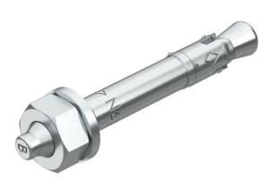
The nail anchor N can be used for multiple fastenings of non-load-bearing systems and in cracked and non-cracked concrete, thereby combining the benefits of a bolt tie with even easier mounting.
