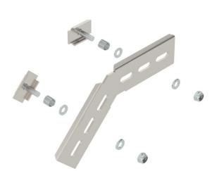
$45^\circ$  installation profile, vertical, for C mesh cable tray and GR-Magic® mesh cable tray with a side height of 55 mm. Each with two clamps of type KS 23 35. Including connector, to create  $45^\circ$  bends.
