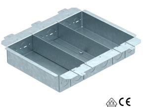
Closed mounting support for receiving 3 APMT5 cover plates. The mounting support is fastened below the GES9DB service outlet. Each with 6 knock-out openings M20 and M25 for the mounting of flexible installation hoses.
