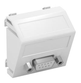
Multimedia support with one D-Sub9 connection socket, slanting cable outlet, with labelling panel, D-Sub9 socket (RS232) with screw connection. Support plate with locking fastening, suitable for horizontal and vertical installation in the system environment.
