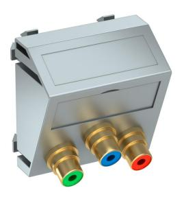
Multimedia support with three cinch connection sockets for component video, slanting cable outlet, with labelling panel, three cinch sockets (RCA) with soldered connection, colour coding red / green / blue. Support plate with locking fastening, suitable for horizontal and vertical installation in the system environment.
