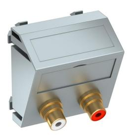
Multimedia support with two cinch connection sockets for audio R/L, slanting cable outlet, with labelling panel, two cinch sockets (RCA) with soldered connection, colour coding red/white. Support plate with locking fastening, suitable for horizontal and vertical installation in the system environment.
